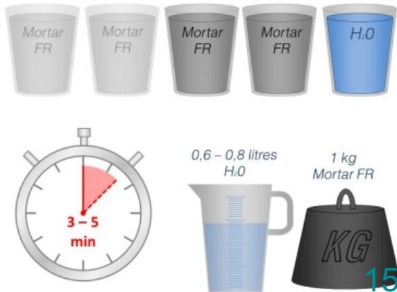
Mixing ratio by weight, mixing time 3-5 minutes:
