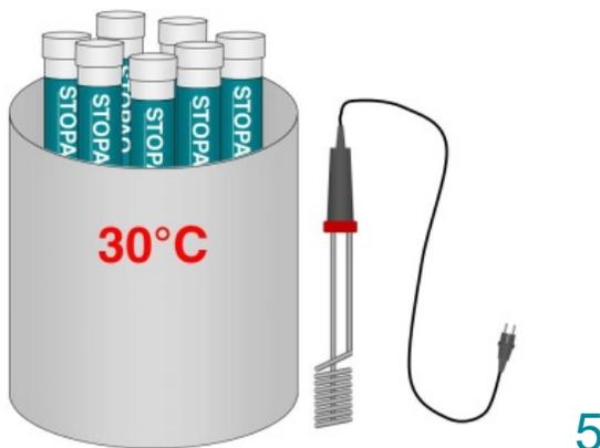
5 Preheat the 2100 Aquastop up to a temperature 30°C. A bucket of water and a water heating coil can be used.
