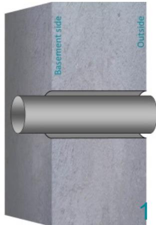
1 Duct to be sealed with a barrier, 2100 Aquastop and Stopaq Mortar FR or WR.
