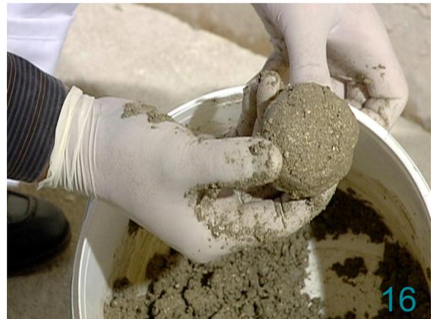
Mortar FR must be used in fire rated walls and floors. Check the malleability of the Mortar FR-WR by moulding the Mortar to a ball shape without it falling apart.
