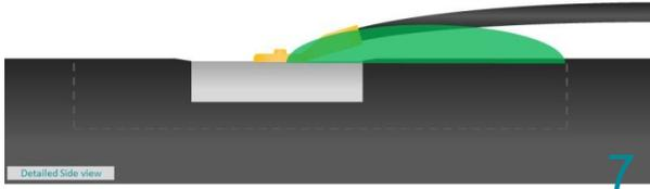
Apply preheated Paste around the Pinbrazed and underneath the connecting wire. Check the adhesion of the paste
